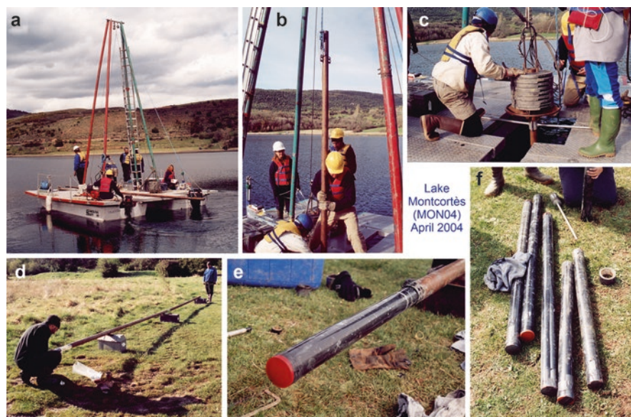
Fig. 4 First coring campaign of Lake Montcortès sediments (April 2004). (a) General view of the LRC coring platform. (b) Dropping the Kullenberg corer until the surface of lake sediments. (c) Loading the cap of the Kullenberg corer (400 g). (d) Full sediment core. (e) Extracting the plastic (polycarbonate) core sediment from its metallic casing. (f) Cut core ready to be transported to the laboratory for analysis. Photos: V. Rull
